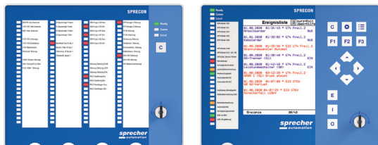
SPRECON-E-CP HMI control panel with event list
