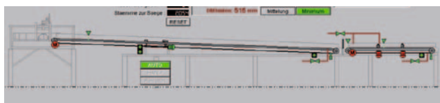
Visualisation of conveying line for log turning
