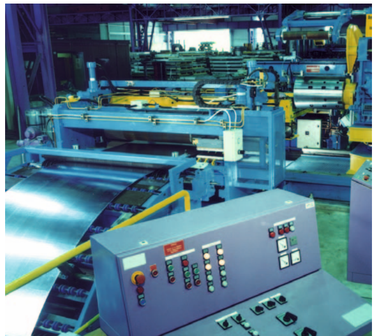
Control console before loop
